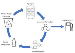
Fig. Plastic Recycling Via Pyrolysis.
