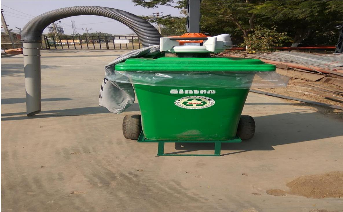
**(Plastic Bag Pickup Machine: Developed by BEIL & SRICT)**
