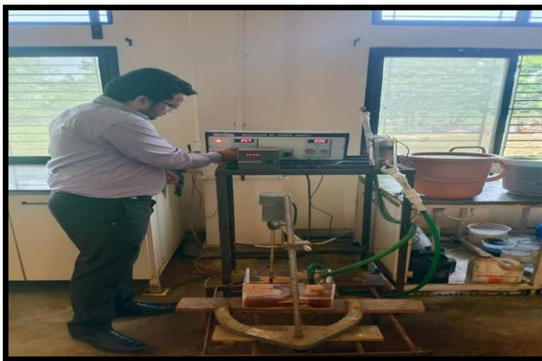
Demonstration of electrochemical oxidation setup
